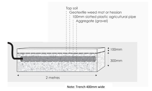
Requires: .3 metres of aggregate 2 metres of 100 mm slotted PVC 2metres of Geotextile cloth
