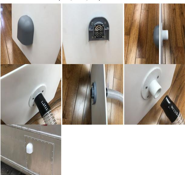
A thin walled structure may not have any way for a PVC pipe to hold through the wall so we recommended using our white hose flange that comes with the toilet in the small parts bag.
